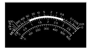
MJ10 scale is shown. BM12 scale is the same but has a battery condition indication mark added.
